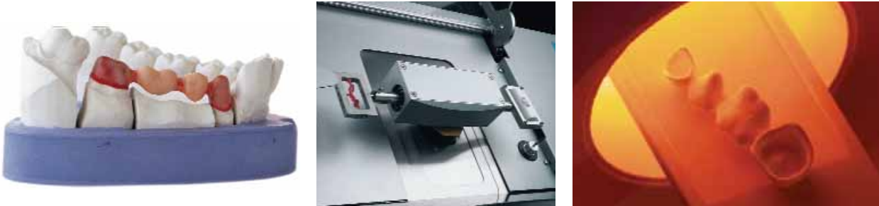
Fig. 6: : Wax Model, Cercon milling in the Brain, and framework being sintered.
