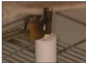
Insert the Ingots and Plunger*
