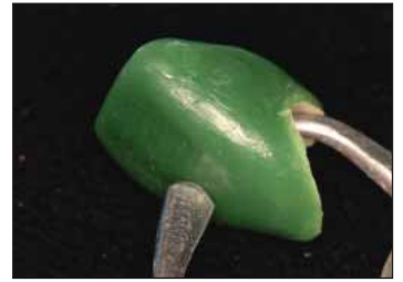
Minimum Wax Thickness of 0.8mm
